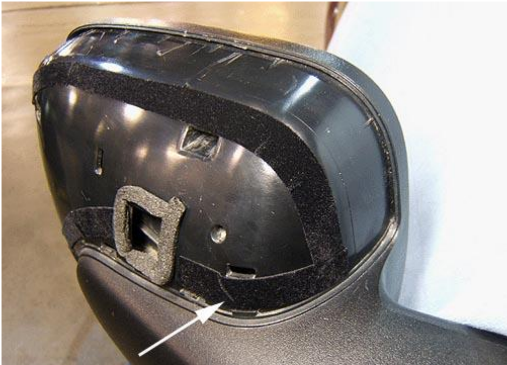
Fig. 5: Locating Another Piece Of Flocking Tape Courtesy of GENERAL MOTORS CORP.
