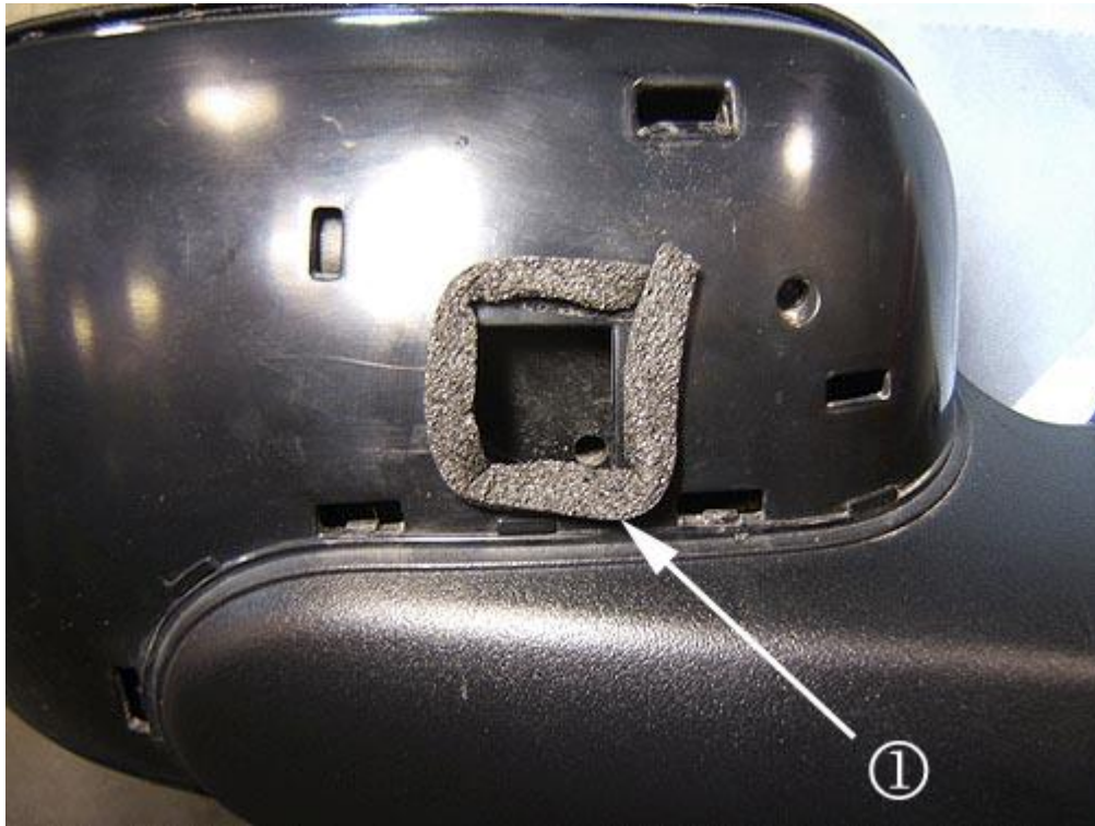
Fig. 3: Locating Adhesive Back Shim Stock Courtesy of GENERAL MOTORS CORP.
