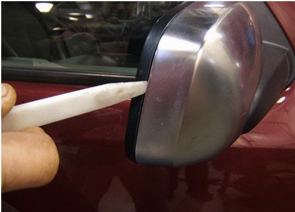
Fig. 1: Removing Outside Rearview Mirror Cover Courtesy of GENERAL MOTORS CORP.
