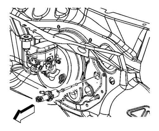
Fig. 2: Clutch Master Cylinder Courtesy of GENERAL MOTORS CORP.
