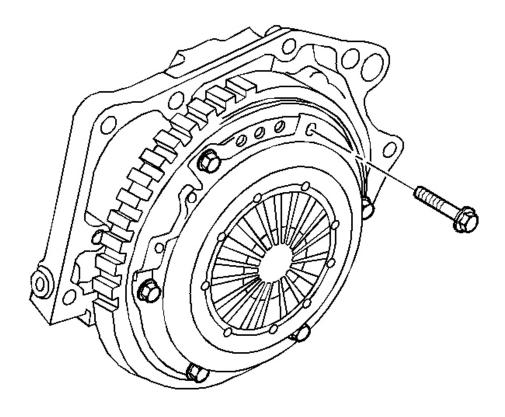
Fig. 8: View Of Clutch Cover Bolt Courtesy of GENERAL MOTORS CORP.
