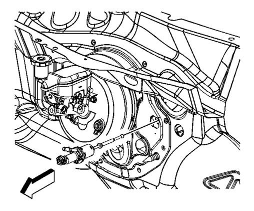
Fig. 3: Clutch Master Cylinder Courtesy of GENERAL MOTORS CORP.
