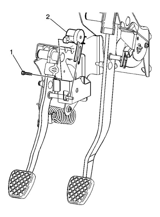
Fig. 7: Clutch Pedal Position Sensor Courtesy of GENERAL MOTORS CORP.
