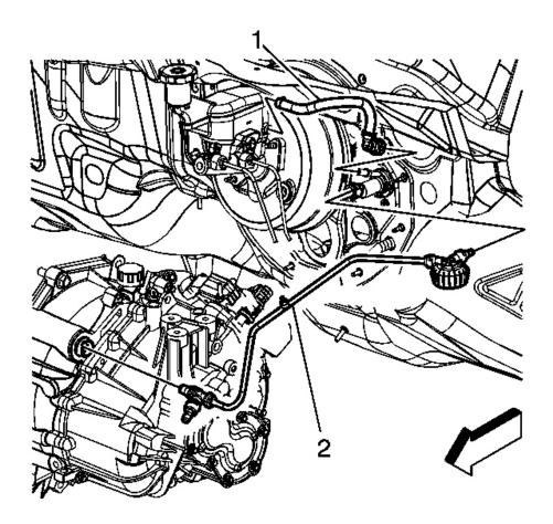
Fig. 6: Clutch Line To Clutch Master Cylinder Courtesy of GENERAL MOTORS CORP.
