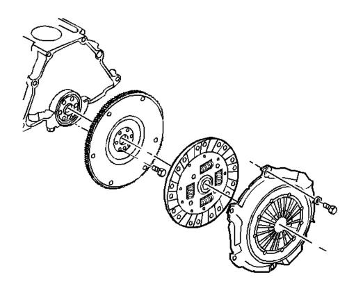
Fig. 9: View Of Clutch Cover And Clutch Disc Courtesy of GENERAL MOTORS CORP.
