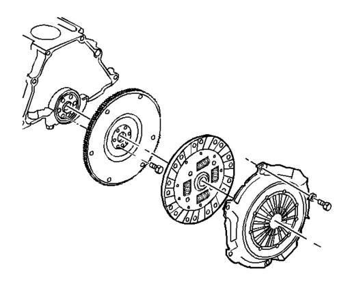
Fig. 10: View Of Clutch Cover And Clutch Disc Courtesy of GENERAL MOTORS CORP.
