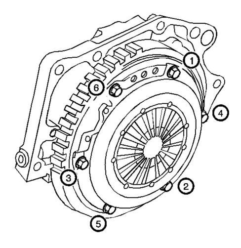
Fig. 12: Locating Clutch Cover To Flywheel Bolts Courtesy of GENERAL MOTORS CORP.
